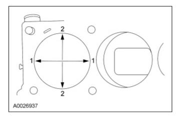
2. **NOTE:** For precision fit, new pistons are divided into 3 categories within each size range based on their relative position within the range. A paint spot or specific size grade on a new piston indicates the position within the size range.
